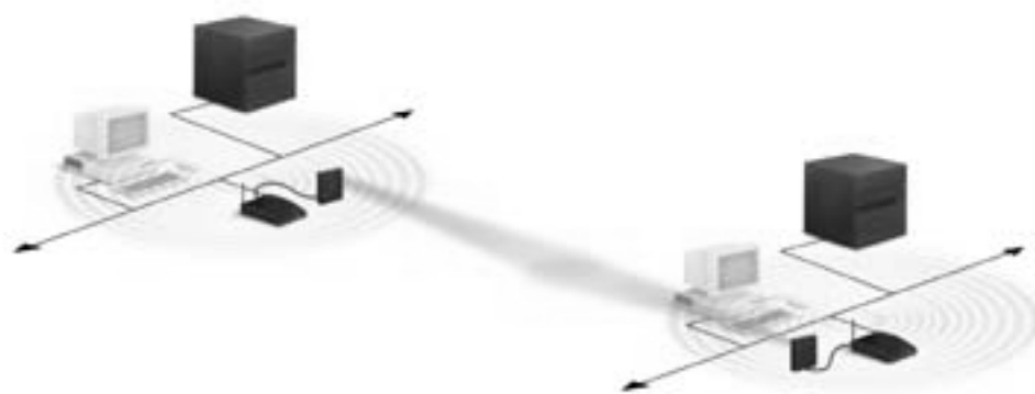
Fig 1.5 The use of directional antennas
