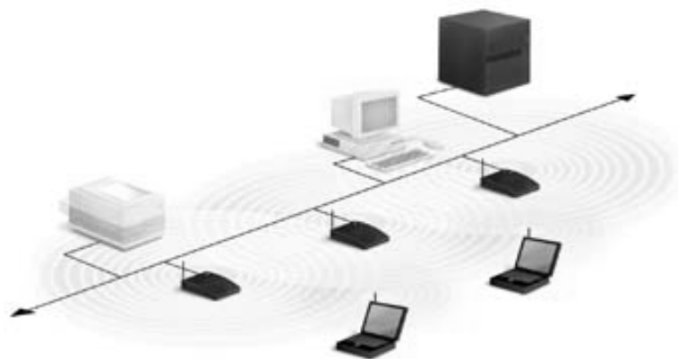
Fig 1.3 Multiple access points and roaming
