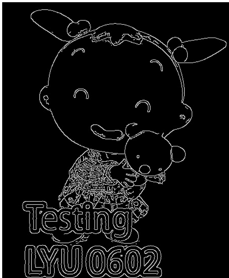
Fig3.5a shows image produced by Canny Edge Detection
