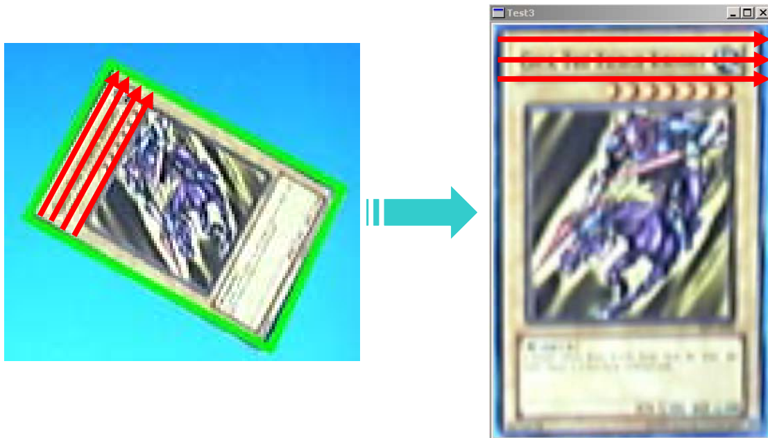
Figure 28: The distorted card image (left) and the resulting undistorted card image (right).
