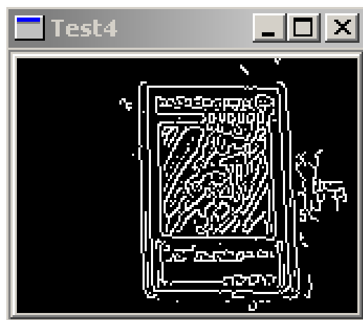
Figure 22: Resulting image after applying Canny algorithm.
