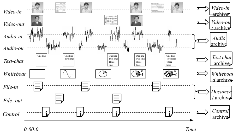
Figure 3.4 Illustration of the logical channels and media
