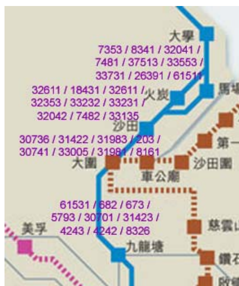
Fig 8.8: Cell IDs of KCR stations for SmarTone between Kowloon Tong station and University station
