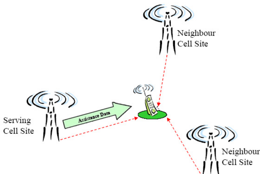
Fig 4.8: GSM E-OTD in operation
