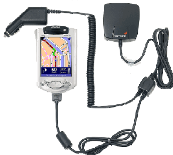
Figure 4.3: PDA equipped with GPS receiver for location determination
