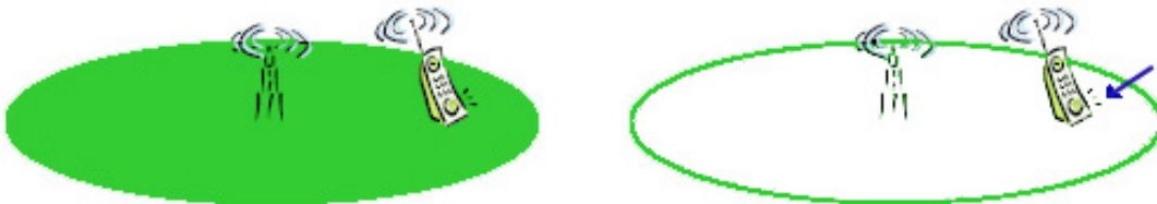
Fig 6.5: The positioning region that two approaches would indicate: pure cell ID detection (left) and cell change method (right)
