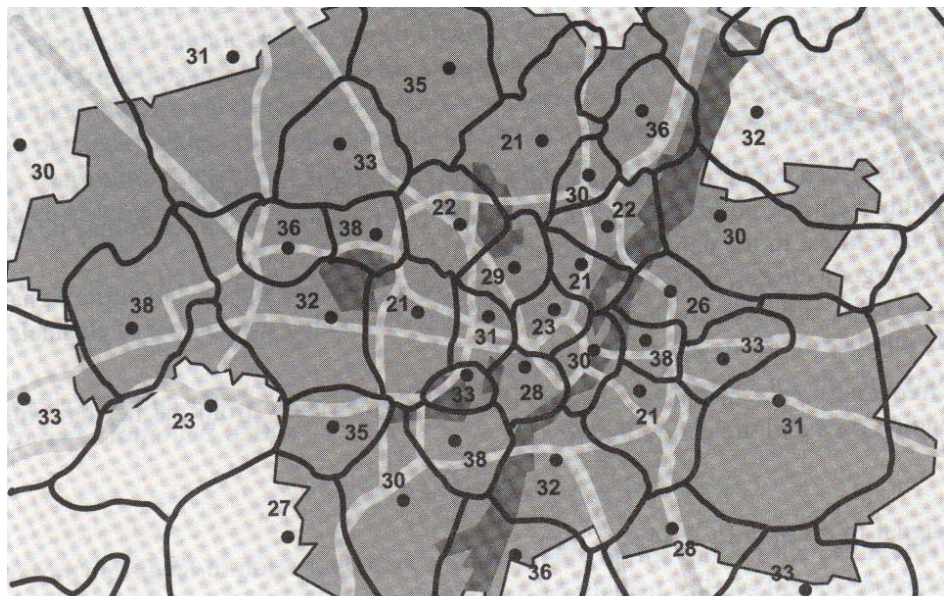
Figure 5.1: Area covered by cells. The dots inside cells represent the base stations
