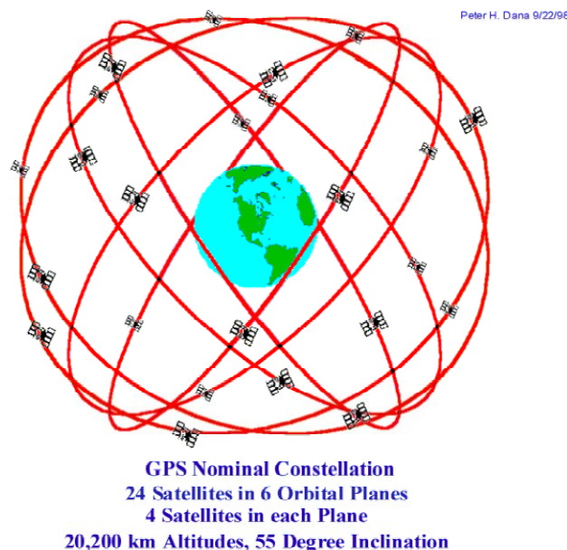
Figure 4.1: 24 satellites and 6 orbital planes for GPS system
