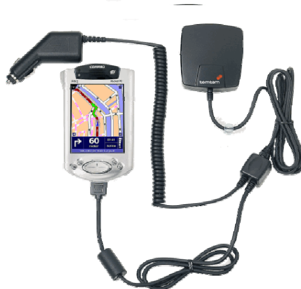
Figure 4.3: PDA equipped with GPS receiver for location determination
