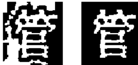
Figure 4.10 Image before (left) and after (right) morphological filtering.
