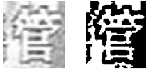
Figure 4.9 Image before (left) and after (right) binarization.
