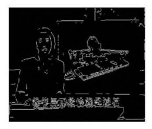
Figure 2: Frame edge filtered by Sobel filter
