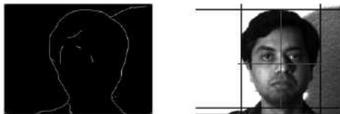
Figure 6.8: Binary image (left) and face region (right)
