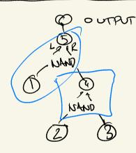
AS A COLORING PROBLEM VERTICES = GATES EDGES = WIRES
