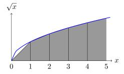
Indeed, the shaded area can be calculated by adding the areas under the first n trapezoids to obtain
