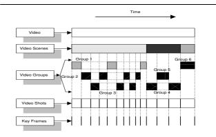
Figure 3. Hierarchical video structure
