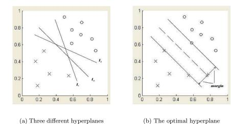
Figure 2.1: Illustration of linearly separable cases of SVM
