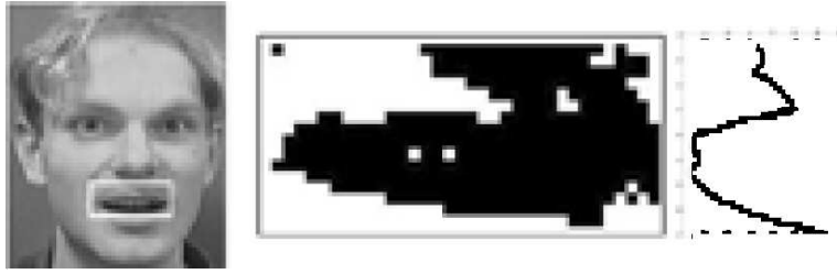
Figure 4.12: The calculation of the mouth position. The extracted mouth region (left), the binary image of mouth region (center), and vertical projection of the binary image (right).
