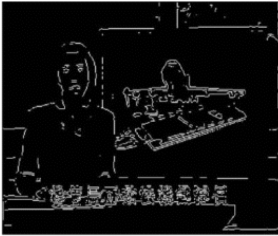
Figure 2: Frame edge filtered by Sobel filter
