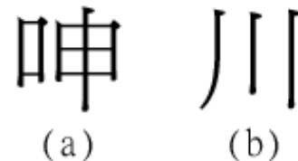
Figure 4: Some Chinese characters would be wrongly regarded as two characters (fig. a) or three characters (fig. b) in vertical projection
