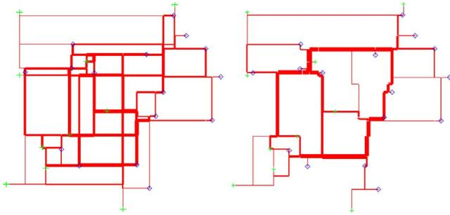
Fig. 14. Case  $T_8$ 's data wires under minimal power and minimal wire.
