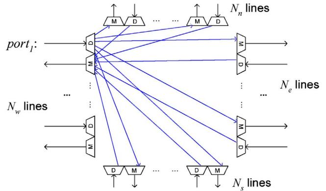
Fig. 13. Implementation of a crossbar switch.
