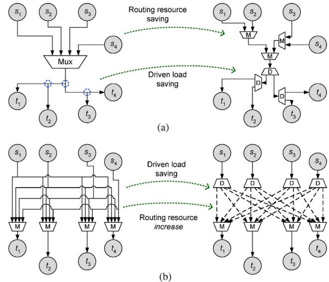
Fig. 3. Bus gating using distributed mux and de-mux. (a) On single bus. (b) On bus matrix.
