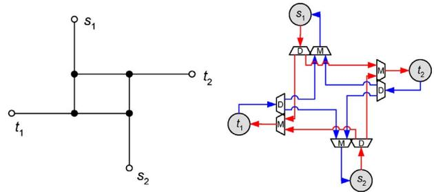
Fig. 4. Shortest-path Steiner graph  $G''$  and its bus implementation.
