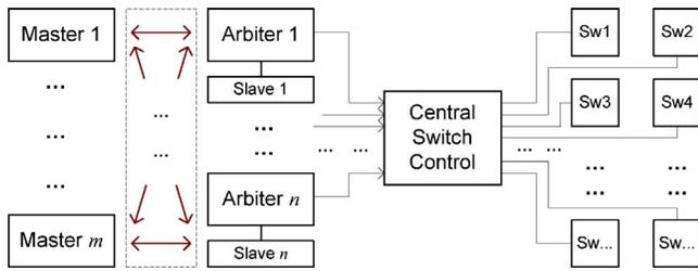
Fig. 12. Control on switches in a bus matrix.
