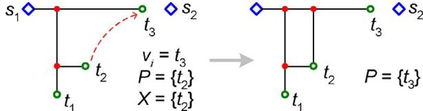
Fig. 7. Connecting a node into the Steiner graph.
