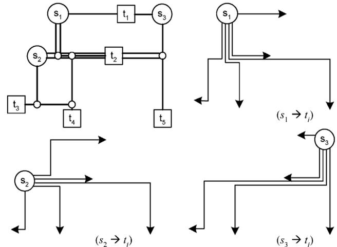
Fig. 8. Bus matrix graph and all its master-slave connections.
