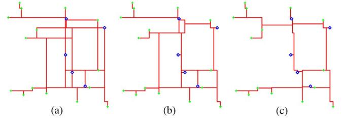
Fig. 10. Merging parallel segments in a bus matrix graph. (a) Original. (b) Reduced. (c) Further reduced.
