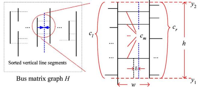
Fig. 11. Searching for mergeable parallel segments (in vertical direction).
