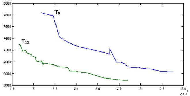
Fig. 15. Average path length versus total (data) wire length in case  $T_8$  and  $T_{12}$ .
