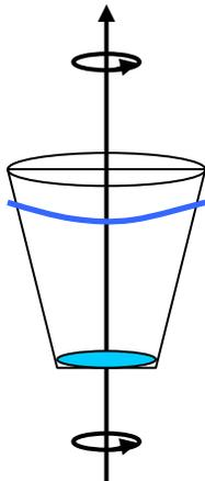
Water surface curved when the bucket is rotating.
